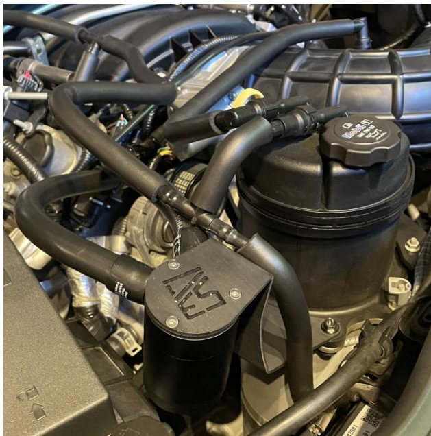
2014 – 2015 Camaro Z/28 Catch Can Kit Installed
