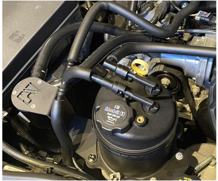
Catch Can Kit Installed
