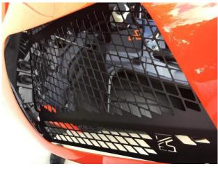
Driver Side Shield Installed
