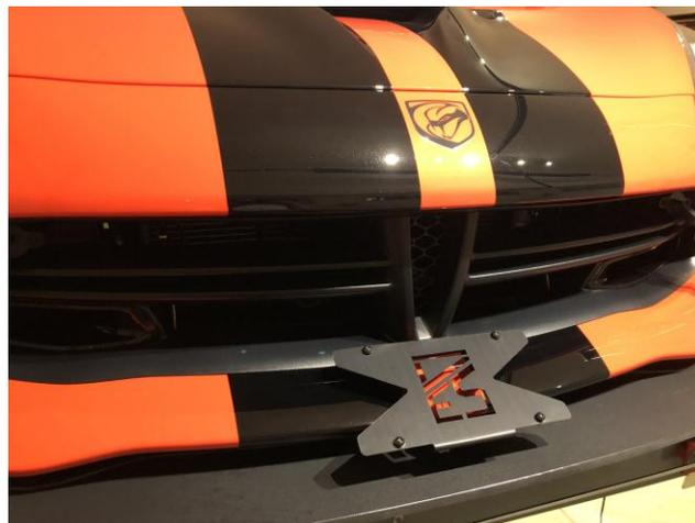
***DSE ACR-E Driver Side Splitter Support Bracket Assembly***
