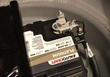
Rear View of Battery and Recommended Strain Relief for Ground Wire
