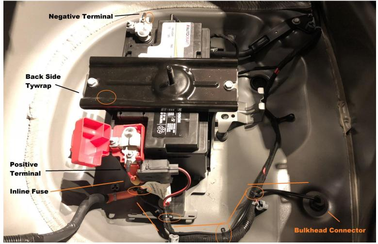
Wiring diagram guide showing routing and ty-wraps (circles). Using this guide, lay wires as it makes sense for your car.
