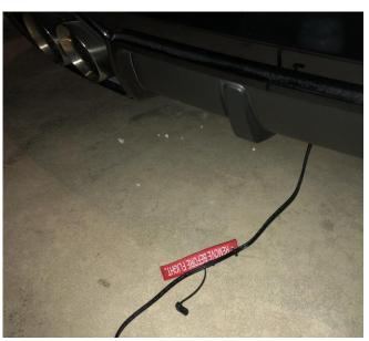
Charging the Battery Through the DSE Quick Access Charging Harness
