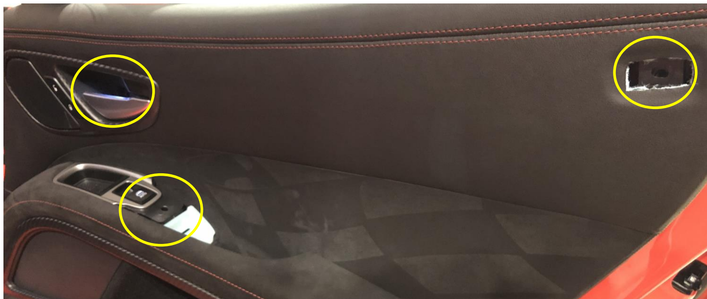
Gen 5 Door Panel Bolts on a 2017
