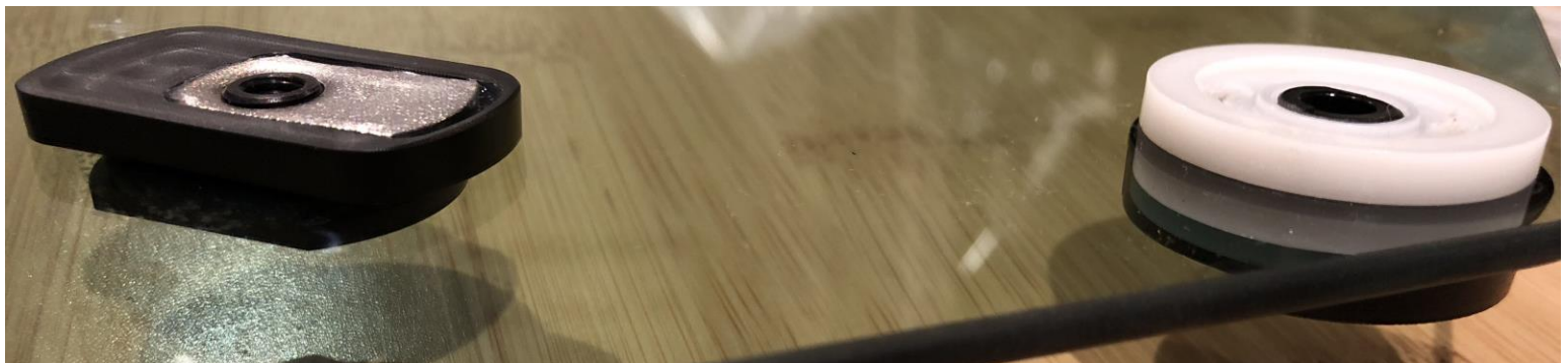
DSE (Left) vs. OEM (Right) Window Boss, inside of window facing upward
