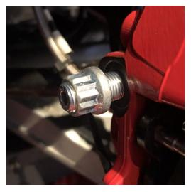
**Nut Installed before Tightening**
