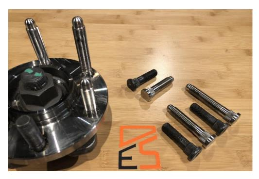
Studs of each length installed on a Viper hub aside OEM studs for comparison
