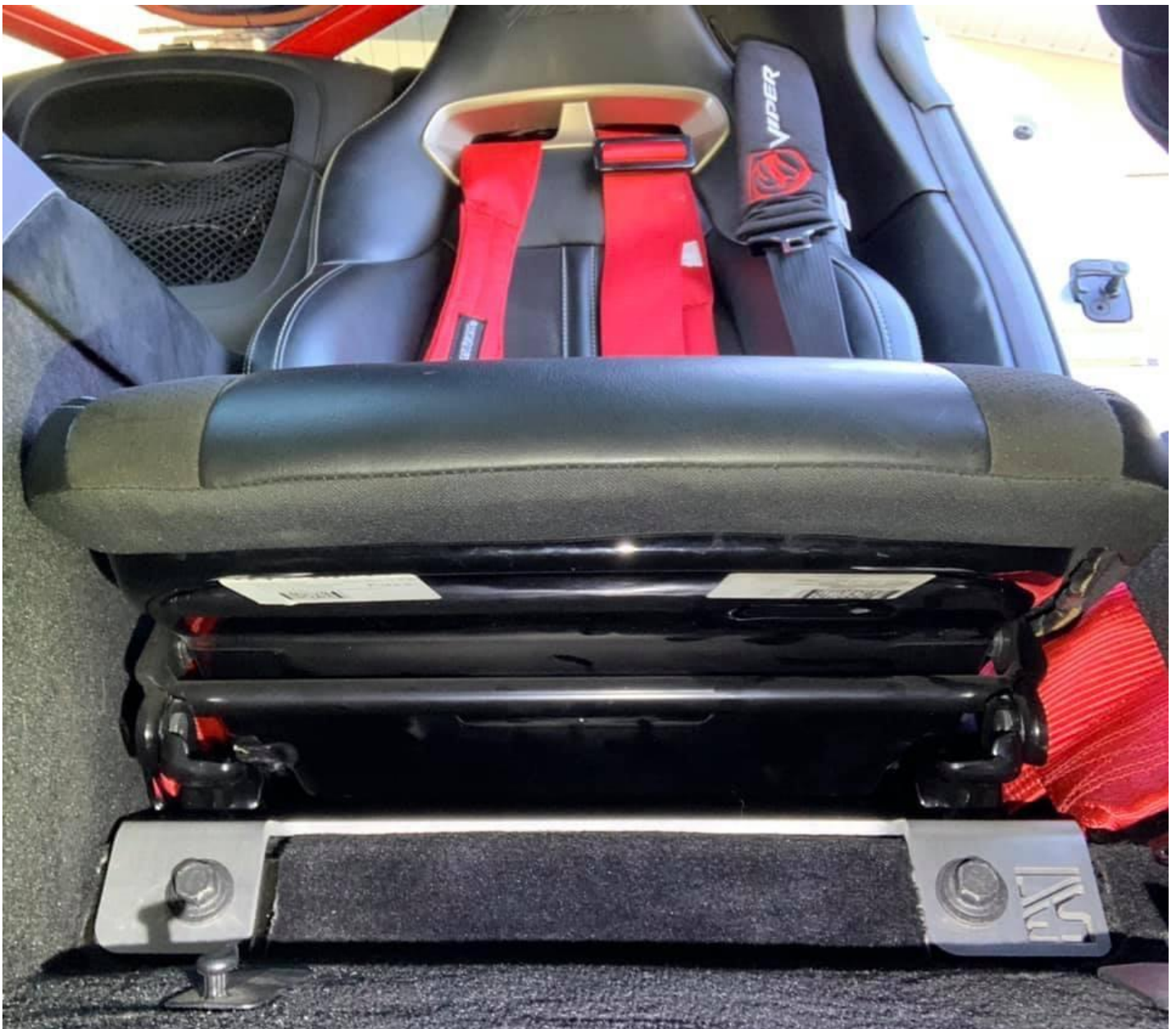
OEM Seat Installed On Lowering Bracket
