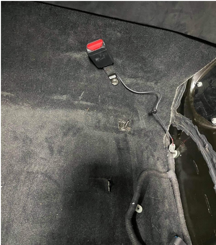
Driver Side Belt Buckle Installed and Wiring Harness Moved
