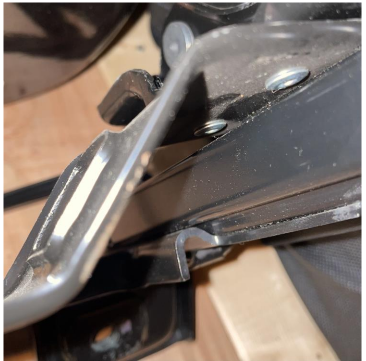
2 Rivets Hold the Crossbar On Each Side
