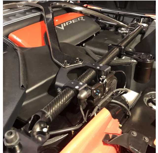
Passenger Side Lateral Carbon Fiber Engine Brace Installed
