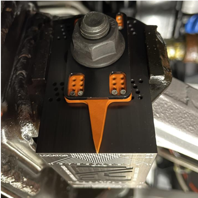
Camber Block Installed
