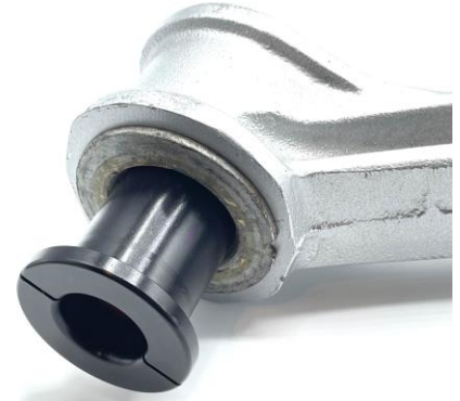
Pressing the Assembly Into the Control Arm
