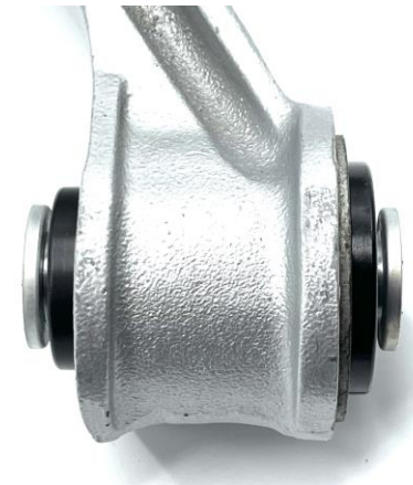
Steel Bushings Pressed into the Moonball
