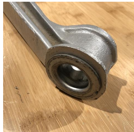
Control Arm Prepared for Bushing Installation
