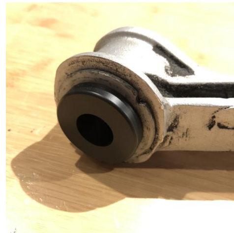
Delrin Bushing Installed
