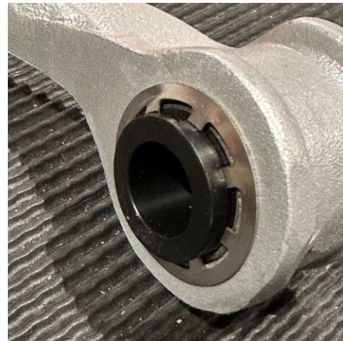
Delrin Bushing Installed with Retainer
