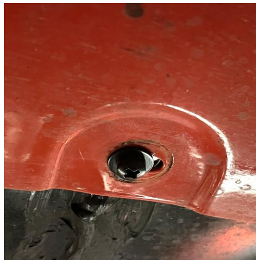
Sill Installed Using New Hardware
