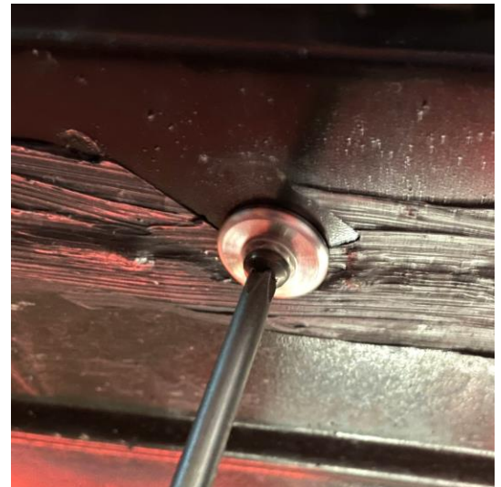
Tighten the sill boss using the Included Hardware
