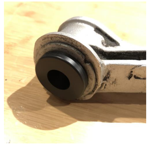
Delrin Bushing Installed
