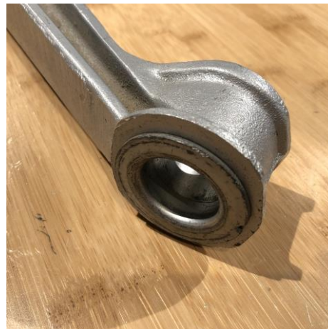
Control Arm Prepared for Bushing Installation
