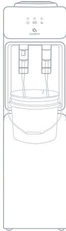
6. After draining is complete, replace the drain cover and use the machine as normal.
