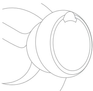
2. Vertically insert the bottle into the bottle supporter (#1) on the top of the machine. The bottle supporter has a built-in puncturing rod to allow you to use spill proof caps without opening the plastic bottle seals.
