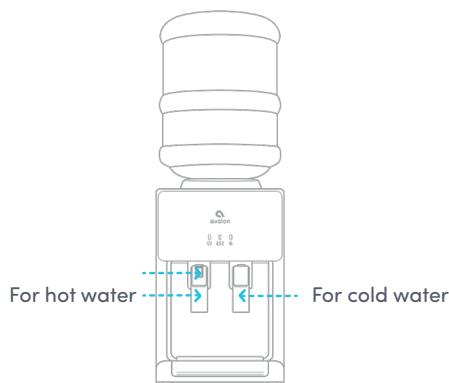
4. Once water is dispensing from both spouts insert the power plug into a power socket. Turn on (I) the heating switch (#13) and the cooling switch (#14). (If you do not wish to have hot water, please leave the heating switch (#13) in the off (O) position. If you do not wish to have cold water please leave the cooling switch (#14) in the off (O) position.)
