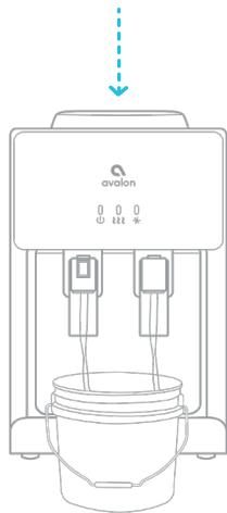
4. Place a large bucket beneath the drain outlet (#12) located on the back of the unit. Remove the drain cover and plug and allow the water to drain from the unit. Water will start flowing as soon as the drain cover is removed.
