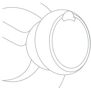
2. Vertically insert the bottle into the bottle supporter (#8) on the top of the machine. The bottle supporter has a built-in puncturing rod to allow you to use spill proof caps without opening the plastic bottle seals.
