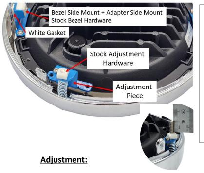
Step 4a: Add the M2.5 screw with Loctite to the Adjustment
