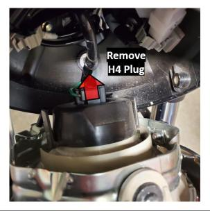
**Step 2:** Remove the headlight assembly. Then unplug the H4 plug powering the headlight.
