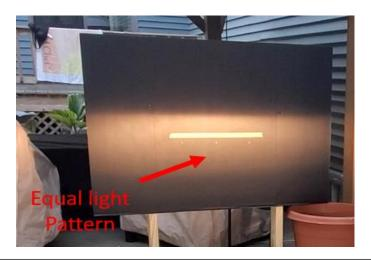
**Adjustment:** After the headlight is installed on your bike position the bike 10 feet from a blank wall. Measure from the ground the height of the headlight (to center) with the rider sitting on it. Now mark your wall with this dimension. Adjust the headlight until the low beam pattern is equally spaced over the line on the wall. The horizontal adjustment should be Neutral to slightly pointed toward the edge of the road away from oncoming traffic.
