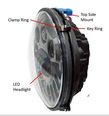
**Step 3a:** Position the top of the Headlight adapter as shown with the top of the Bezel. Work the top of the adapter in first on an angle and then slide the back in. [Optional: If having issues at this point one of the side mounts can be removed until you get the assembly in the bezel. Then add the side mount back.]
