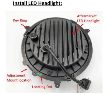
**Step 1:** Take the Key Ring and align the three keyways and keys of the LED headlight. The LED headlight should be facing up and the adjustment mount location to be positioned to the bottom left. A colored locating dot should be visible.
