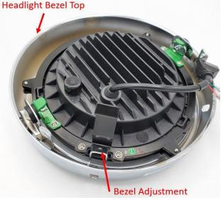
**Step 5:** Slide the headlight assembly in the Suzuki bezel from the back side (top to bottom). Line up the side mount holes with the bezel mounts. Use the existing hardware from the stock headlight. Have the T-Nuts facing each other. You can use Blue Thread Lock on the
