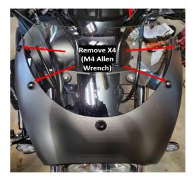
**Step 1 (Optional):** Remove any cowl or fairing that may get in the way of the headlight bucket screws in step 2. Hardware may vary.
