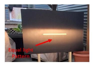
**Adjustment:** After the headlight is installed on your bike position the bike 10 feet from a blank wall. Measure from the ground the height of the headlight (to center) with the rider sitting on it. Now mark your wall with this dimension. Adjust the headlight until the low beam pattern is equally spaced over the line on the wall.
