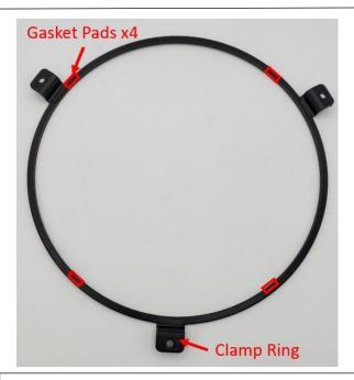
**Step 2:** Apply the 4 provided EPDM gasket cutouts to the bottom side (tabs facing up) of the clamp ring in the approximate locations described above. This will cushion the LED headlight in the setup and reduce vibration. When applying use pressure for 20 seconds. This is an optional step but will reduce shifting of the light.
