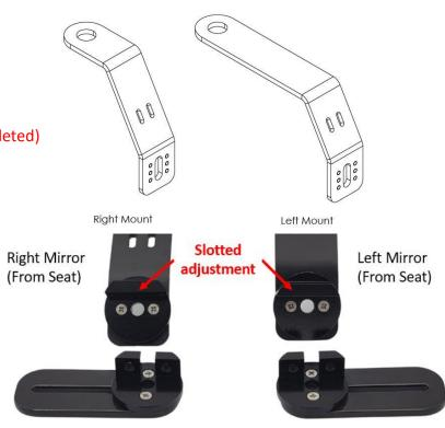
**Step 3:** Assemble the Left and Right mounts with their respective Center Mounts. Use the M5 screw, M5 washer and Nylock nut (no Loctite required here). Do not tighten all the way. The M5 washer goes on the head side of the screw to reduce the length of exposed screw.
