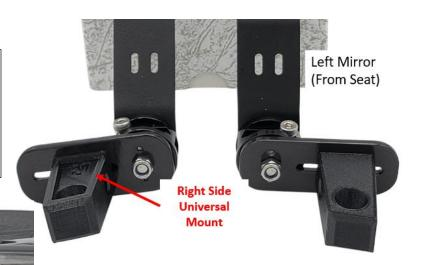
**Step 5:** Attach the PowerMadd Handguards to the mounts using the M6 screw and Nylock nut (No Loctite required). The screw head should be facing toward the rotating adjustment hub. Tighten the nut until it is snug. Do not overtighten.
