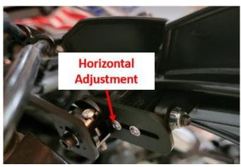
**Step 8:** Move the Universal Mounts to a location that makes both left and right sides equally spaced when viewing from the center. Tighten the M3 screws. Do Not Overtighten.
