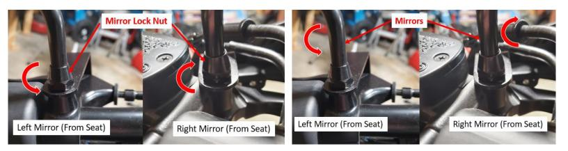
**Step 1a:** Loosen the left mirror nut with a M17 wrench. Loosen CCW. Once the nut is released the mirror also loosens CCW by hand. Remove the mirror. **Do not strip the threads on the mirror or nut.**  **Step 1b:** Loosen the right mirror nut with a M17 wrench. Loosen CW. Once the nut is released the mirror also loosens CW by hand. Remove the mirror. **Do not strip the threads on the mirror or nut.**
