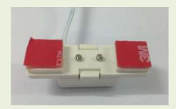
3. When the sensor probe detects a leak, the flood sensor device will send an "alarm" message.
