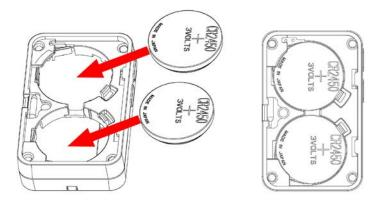
Note: To install the battery, use a screwdriver or similar tool to assist in opening the battery cover.
