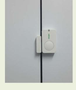
Places which are necessary to detect the opening and closing state
