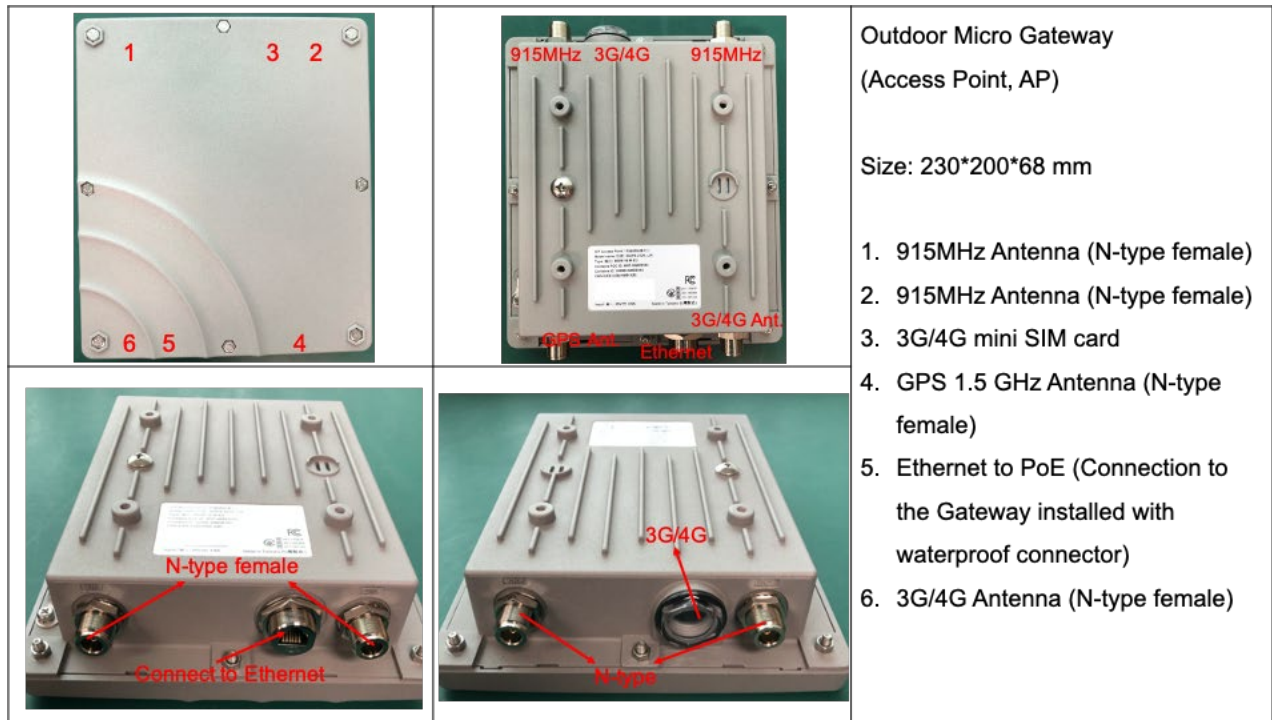
Figure 5 Gateway Installation Instructions
