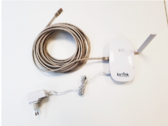
Ethernet cable, power supply and LoRa antenna connections
