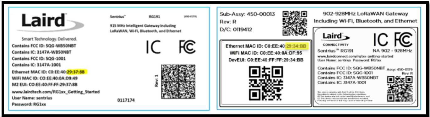
Figure 7: Determining the gateway Ethernet MAC address
