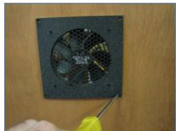
Measure the exact cutout size you need to install the bracket. The size will be noted on the product information sheet and on our website. Attach bracket to cabinet using the enclosed wood screws. Connect fan to power source or thermal controller.
