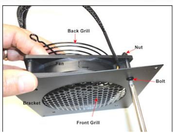
(2) Using the Nut and Bolts attach the grills to the fan and bracket by sliding bolt through bracket then front grill then fan and back grill. Then attach nut to bolt. Repeat on each corner of fan. Direction of air flow can be changed by reversing position of fan before attaching to bracket.
