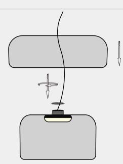
2. LED bulb crosses through the hole of the second layer shade, put the second gasket then tighten it.
