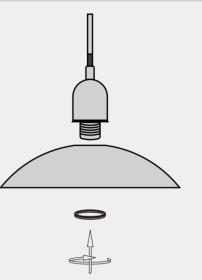
Fix the lampshade with the locking plate.
