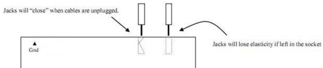
If jacks are damaged or left in the open position, the internal probes will not engage when testing for surface resistivity.
