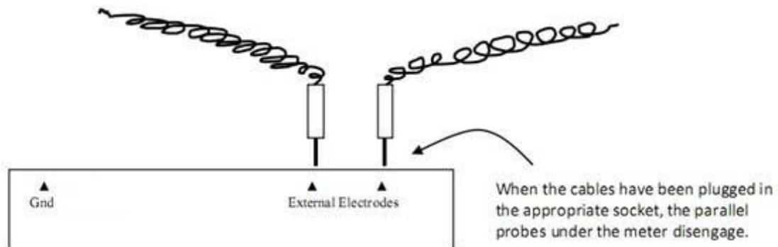
Attach one lead to a 5 lb probe and place probe on the floor that's being tested.
