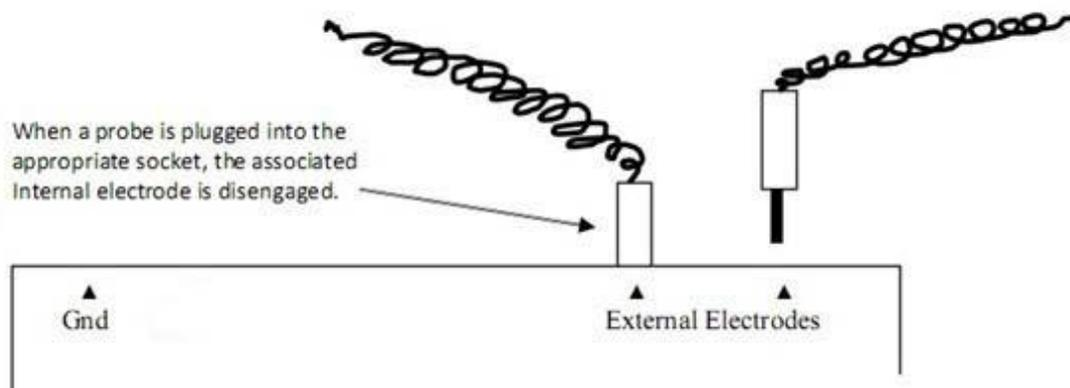
By utilizing these probes to the S2020RHR's sockets it is possible to measure Point to Point (RTT) Resistance, Surface to Ground (RTG), and Volume Resistance. Using these probes will allow compliancy with various standards including ANSI/ESDA S4.1 for Worksurface - Resistance Measurements, ANSI/ESDA S7.1 Resistive Characterization of Materials - Floor Materials.
