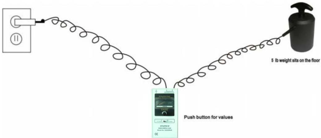
AN EXAMPLE OF MEASURING RTG ON DISSIPATIVE TABLE MATS:
