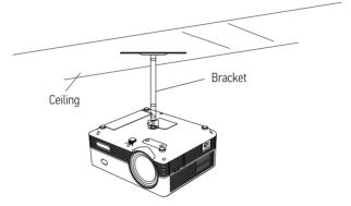
When ceiling mounting the projector, please ensure screws of a suitable quality are used, and that screw depth is deep enough to prevent the projector from falling.
