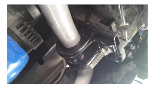
**4.** Next will be attaching the endlinks. I replaced mine with the RTR Tactical adjustable endlinks. *They are available at americanmuscle.com, and are significantly better than the factory endlinks*. The stiffest setting on the bar is the hole furthest from the end of the bar. This picture is of the second loosest setting. All endlink nuts should be tightened to **85 ft/lbs.**
