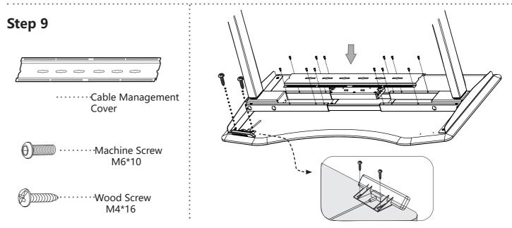
Place the **Cable Management Cover** on top and insert **twelve(12) M6\*10 Machine Screws** partially.
