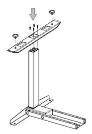
Loosely attach a **Foot** to the bottom of each **Lifting Column** using **four (4) Machine Screws** per Foot. Once all the screws are in place, tighten them down the rest of the way.
