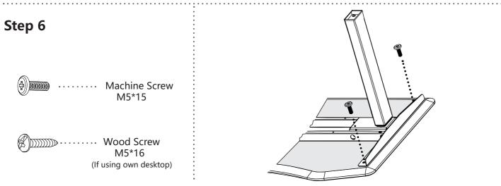
Secure the other Leg Assembly to the desktop with **two(2) M5\*15 Machine Screws** or M5\*16 Wood Screws (if using your own desktop).
