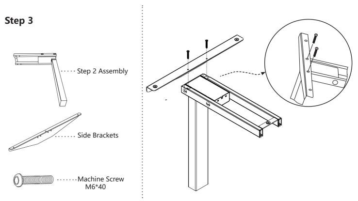
Hold up the assembly from Step 2 as shown. Insert **two(2) M6\*40 Machine Screws** through the two(2) holes of the **Side Bracket** going into the **Crossbar End** assembly.
