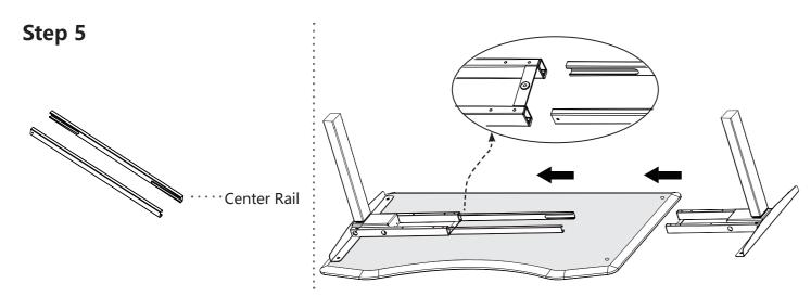
Slide the **Center Rails** into the **Crossbar End** attached to the desktop as shown, so that the cut-out slots are facing inwards.
