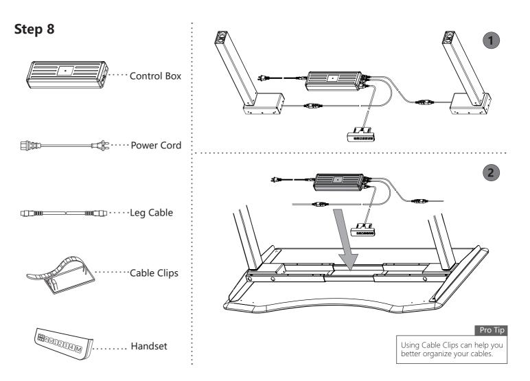
As shown in Figure 1, connect the **Leg Cable** to the lifting column and the Control Box. Connect the **Handset cable** to the Control Box.
