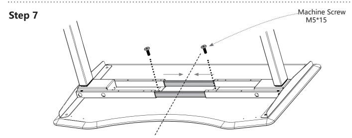
Slide each Center Rail until the center indicator mark light marking is in the middle.
