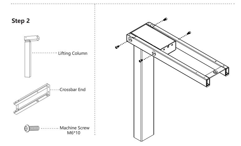
Insert one of the Lifting Columns (either one; they're identical) into the Crossbar End.
