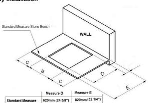
MODEL MEASURE B MEASURE C 585mm 23" 550mm 21. 5/8" >= 100mm 4" 785mm 30. 7/8" 750mm 29. 1/8" >= 100mm 4"
