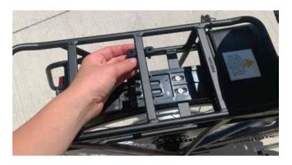
5. Place Carrier on top of middle bar so that the two screw-holes are lined up with those on the grip underneath
