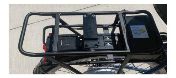
7. Repeat steps 4 and 6 by placing the second Foot Bracket underneath the middle bar, lined up with the Carrier, then fasten final two screws in place
