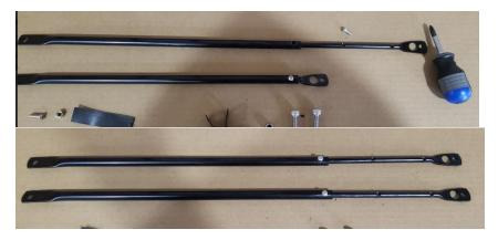
4. Install Strut loops on the bottom of basket using the smaller hole, and secure with smaller screws and nut (Note: Do not fully tighten until the assembly is complete, then make sure to secure)
