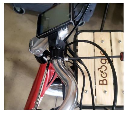
8. Make sure all screws are tight and secured and no wires are pinched. Call Boogie Bikes if you have any questions or safety concerns.
