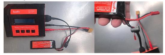
• When charging the Drone battery, please connect the white plug from the charger into the white plug of the battery. The white plugs on the on the battery will match the indent on the charger connector (it will only go one way). Then the YELLOW connector of the Charger connects to the YELLOW connector or the battery.
