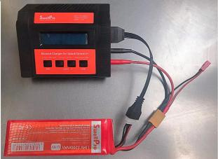
When charging the battery, after plugging In the charger at the wall, power on the charger & plug in both cables to the battery as shown above. After about ten seconds the charger will start automatically.
