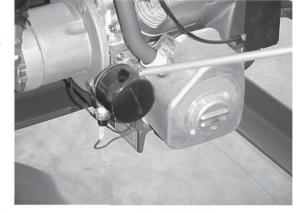
This photo illustrates the Oil filter location on the engine. Replace filter every 6 months for smooth engine operation
