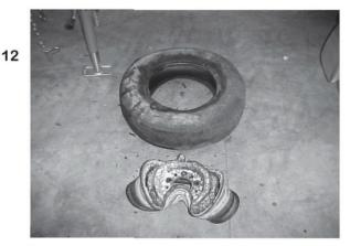
This photo illustrates the wheel crushed and separated from the tire.
