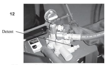
If the valve "kicks out" on the arms return stroke, the detent will have to be tightened slightly.
