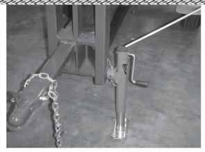
Position TC-300 near tire and wheel supply to be crushed. Place front support jack in position. Crank jack to bring TC-300 main beam to approximate level position.
