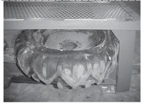
Position tire to the front against the crushing frame as shown.
