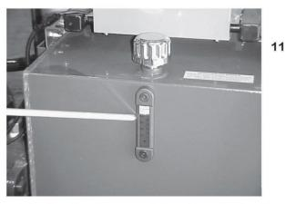
Check hydraulic oil reservoir level by viewing the sight glass. Oil level should be approximately 3" - 5" from the top.
