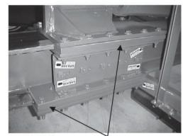
The crushing wedge has space wear bars on both the upper and lower slides. These wear bars may need adjusting. Loosen 6 upper and 6 lower cap screws and slide wear bars up to beam flange. Leave 1/32 clearance between beam and wear bar. If wear bars are worn too much, remove bars and turn side to side. This will give a new side to guide on. DO NOT ALLOW SLIDE BOLTS TO LOOSEN. KEEP BOLTS TIGHT TO 100 FT-LBS & ADJUST SLIDE PLATES IF NECESSARY.
