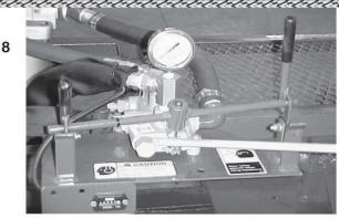
This photo illustrates the adjustment location of the hydraulic pump pressure to the valve. The gauge should read 2800—3000 PSI when the ram is fully extended. To increase pressure, first remove large Hex nut. Then using a Hex Allen wrench—turn adjustment screw to the right 1/4 turn at a time & recheck until pressure is 2800—3000 PSI.
