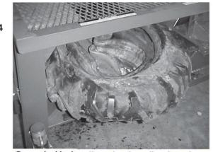
Operate Hydraulic valve handles to return crushing wedge to the starting position.
