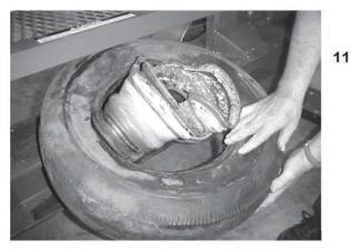
Slide the wheel and tire out of the TC-300 chamber. *NOTE: The wheel & tire can be taken out of either side of the machine*
