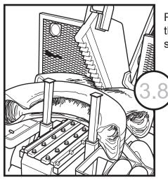
Reposition the push/pull bars after the shear blade returns to the up position. Then reposition both of the tire halves as shown and shear through them as shown.
