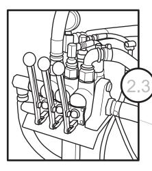
This illustration shows the operating control levers. The left lever controls the shear arm. The center lever controls the tire push/pull bars. The right lever controls the tire lift. Insert the hydraulic push/pull bars into their sockets. Adjust length as required for tire width, either by the ball detent pin or with the adjusting cap screw.
