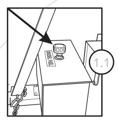
Remove the solid plug in the diesel fuel tank. Fill the tank with #2 diesel fuel at normal temperatures. Insert the vent cap in the tank.
