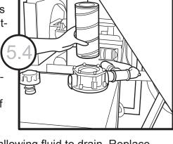
element slowly allowing fluid to drain. Replace with a new element. Replace filter cap and 6 cap screws.
