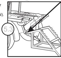
Replace hydraulic filter element every six months or more frequently under heavy use or in dusty climate conditions. Disassemble the 6 cap screws on top of filter assembly. Remove filter
