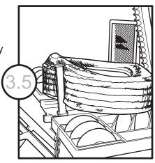
By operating the lever on the left. move shear arm down to begin the shearing process.
