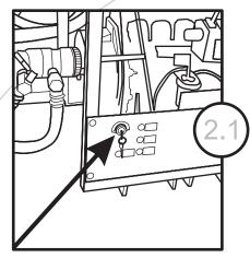
The machine instrument panel, shows the key switch along with indicator lights. Turning the key to the left activates the engine glow plug. Use this position when starting a cold engine. The glow plug indicator light shows the operator when to start the engine.
