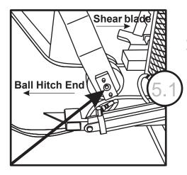
Grease main pivot bearings once a week. There is one bearing on each side of the machine.
