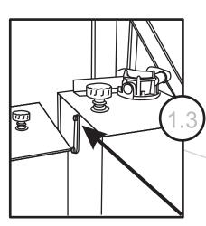
The hydraulic oil reservoir. Should be filled 2 to 3 inches from the top. If you add or change the fluid, use Type A automatic transmission fluid
