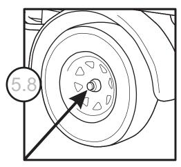
Every six months or prior to towing, remove wheels and inspect hub assemblies. Disassemble the wheel hub assembly and pack grease into wheel bearings and seals if required.
