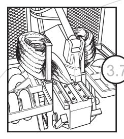
Continue to shear tire all the way through. Some additional adjustment may be done to the push/pull bars during the shearing to maintain pressure or position on the truck tire.
