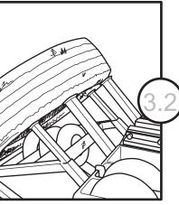
By operating tire lift control lever on the right, the tire is raised to the cutting table.
