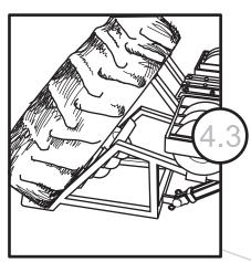
Support the top end of the tire on the push/pull bars. Operate hydraulic lift to raise the tire to the cutting table. The tire should drop over the push/pull bars once raised horizontally.
