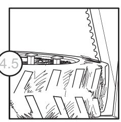
By using the tire cut lever on the left begin to shear tire.
