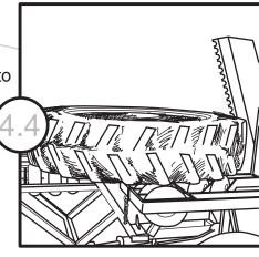
Position push/pull bars against the inside lip of the tire. Do not press the push/pull bars firmly as some adjustment may be required during shearing process.
