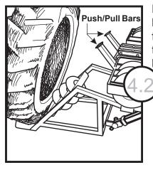
Position push/pull bars as shown here for a large tire. Roll the tire onto the tire lift.
