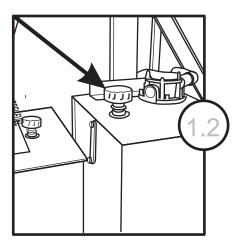
Remove the solid plug from the hydraulic oil reservoir. Insert the vent cap in the hydraulic oil reservoir.
