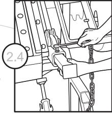
Position stop arms on the lift as required. Insert ball detent pin into stop arm pin holes.
