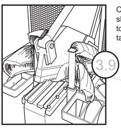
Complete shearing the tire halves. When completed return the shear blade to the up position and the push pull bars rearward to the start position. Remove the cut pieces from the cutting table.
