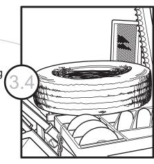
Using center hydraulic control lever, move tire push/pull bars firmly against the tire.
