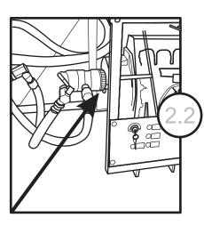
Throttle control increases or decreases engine speed. Turn counter-clockwise to increase and clockwise to decrease.
