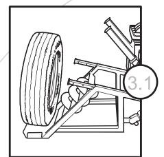
When arms positioned as shown, roll tire on hydraulic tire lift pad. Start engine by following engine operating instructions.
