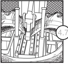
Continue to shear tire, making adjustments to the push/pull bars as required.
