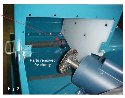
Whether the rim is steel or aluminum, severely corroded to mildly corroded, the applied force of the wire wheel brush contacting the rim needs to be taken into consideration. Too much force could cause damage to an aluminum rim, the unit motor or the wire wheel brush. Too little force will not allow the unit to properly clean a rim.
