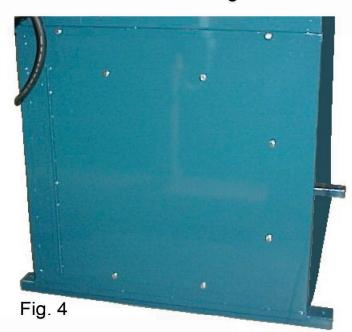
Facing unit an access panel is located to the right. Turn power OFF before opening door.
