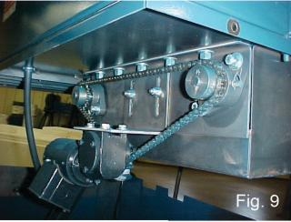
Grease all four bearing zerks as needed. (Too much grease collects dirt.)
