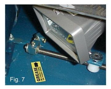
At right are two grease zerks. Lubricate each location.
