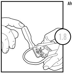
After grooving cutter is installed, tighten locking screws to retain the cutter.
