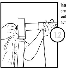
Insert cross arm over vertical arm support — adjust to upper vertical height. Tighten lock nut as shown.
