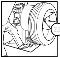
To rotate tire, step on right pedal.
