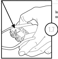
Insert grooving cutter into grooving head. Depending on width of groove desired, a variety of cutters are available. Choose width as desired.
