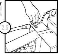
The grooving tool control unit has four heat settings. The left button is the coolest and the right button is the hottest.
