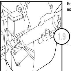
Grease zerks that are marked to grease on a regular basis. Apply light oil to all other moving or pivot points.
