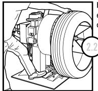
Hold tire in position and activate expanding holding arms by stepping on left foot pedal, marked "Spread Tire". Position tire to the left side of holding arm next to the stop arm.
