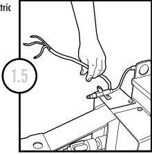
Connect airline to air valve at rear of machine.
