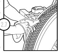
After tire is grooved, it can be removed from grooving stand by releasing the tire holding arms. To release arms lift up left pedal with the toe of operator's shoe. This will release the tire - Shut off air and electric motor until operator is ready to groove another tire.
