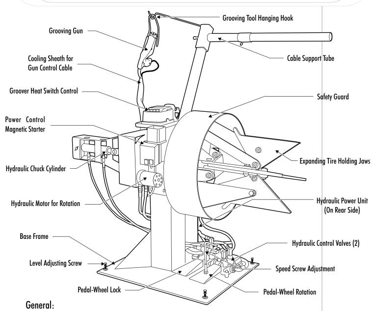
Never wet the motor, electric switch, or components. Cover these items if machine is to be washed. Always disconnect electrical power before attempting any maintenance.
