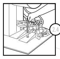
To adjust rotation speed, adjust foot pedal speed control. To slow down rotation, turn speed control clockwise or to the right. To speed up rotation, turn speed control counter clockwise.
