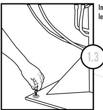
Insert base level screws and level machine.
