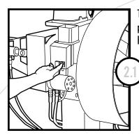
To begin grooving, tire must be placed on holding arms. To activate hydraulic system, push start button.
