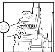
Grasp the grooving tool with cable and roller attached. Step on right pedal to rotate tire. With the air valve on and one button of control unit depressed, position tool and follow existing zigzag pattern. Remove waste as tire rotates. Cross grooves can be cut manually with the grooving tool.
