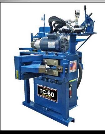
Available in an 3 HP electric motor or 10 HP B&S gas engine
