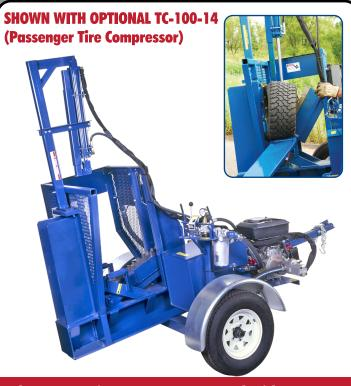
The TC-100 Tire Cutter comes stand with a 18 HP B&S gas engine with electric start. Optional Kubota diesel engine is available
