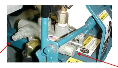
If valve "kicks out" on the shear arm return stoke, the detent will have to be slightly tightened. Tighten outer nut 1/4 turn and tighten lock nut. Continue to cut. If valve still "kicks out" readjust it another 1/4 turn.
