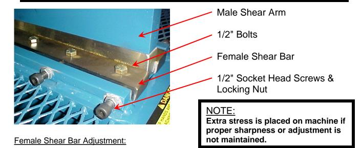
As the steel belting from a tire starts to string out and not cut properly the original bar edges will eventually need to be adjusted.
