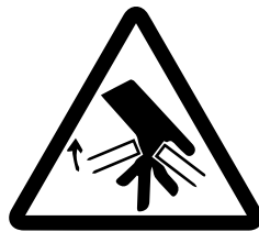
HAND CRUSH/ PINCH POINT
