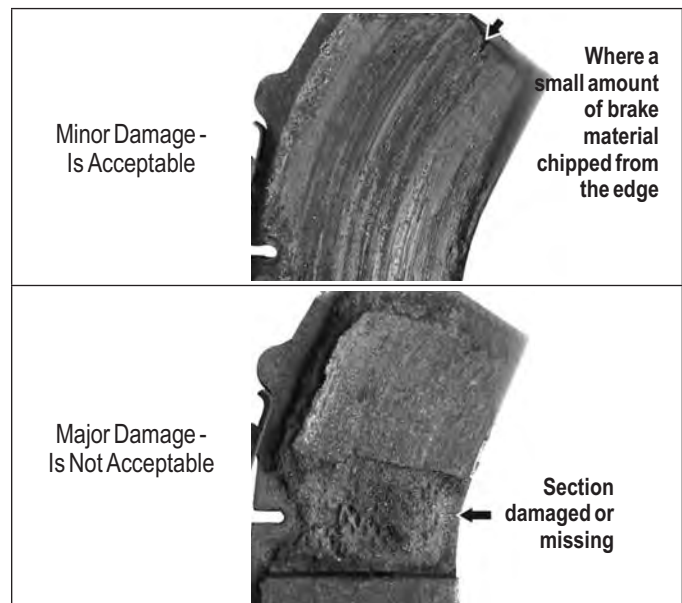
FIGURE 24 - BRAKE PAD SURFACE INSPECTION
