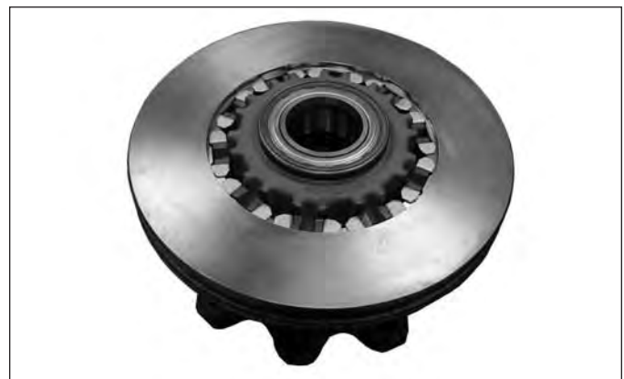
FIGURE 90 - INTERMEDIATE ELEMENTS (SPACERS) INSTALLED
