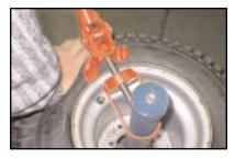
After the guide is properly positioned, hold both handles in your left hand. Push down on the sidewall with your right hand. This provides a "starting place" for insertion of the tool. Raise both handles and slide the toe between the rim and bead. keep your right hand clear of the insertion area to avoid pinching.
