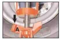
Align the edge of guide (A) with the edge of the outer-flange of the wheel (see above diagram for proper placement).
