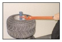
Once the toe is securely placed between the rim and bead, lower the handles to the horizontal position.
