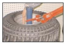
Next, lift the mounting collar and bead breaker off the center-post. Repeat the entire process after the tire has been lifted off the tire-changing machine and opposite side is facing upward.
