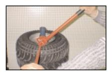
After the top handle has been raised to a vertical position and your left hand has been placed on the bottom handle, pull the black handle grip toward you in a clockwise fashion to about  $45^{\circ}$ . The left hand should remain on bottom handle to provide stability N OT pressure. (This tool can be used in one direction only. You must have the your left hand on the bottom handle and the atv bead braker on the left side of you body during operation).
