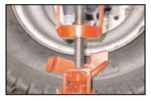
If the guide is not properly positioned (see above diagram), the tool may slip out from under the rim or cause damage to either the bead or sidewall of the tire during use. Once properly adjusted, LUBRICATE THE ENTIRE BEAD AREA (Ken-Tool recommends Bead-Eze). This is particularly important to provide a gliding effect as the bead breaker is moved around the tire, and to prevent damage to the tire.
