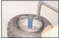
If you are using the Ken-Tool Small Tire Changing Machine, take the Tire Snake and demount the tire.
