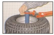
Hold both handles of the ATV Bead Breaker in your left hand. With your right hand, lower the adjustable, mounting collar over the center-post of the tire-changing machine. Hold both handles horizontal and look downward to check the tool alignment.
