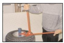
Your **LEFT** hand should be placed on the bottom handle. DO NOT apply much pressure to the bottom handle. If too much force is applied to the bottom handle, bead breaking will be more difficult and damage to the center-post may result.
