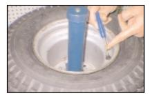
Remove valve core and place ATV tire and rim assembly on any sturdy, center-post, tire-changing machine (we recommend Ken-Tool 38600 or 38601 series). Center the tire and secure the rim to the tire-changing machine.
