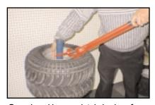
Once bead is completely broken from the rim lock, lift both handles together and disengage the breaker from under the rim.
