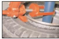
Take note that everything rotates except the mounting collar. This motion pushes the bead below the bead lock on the rim assembly. Relube in to the open gap between the bead and rim.
