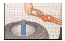
To adjust the breaker, remove the tool from the center-post and rotate the mounting collar. Replace the mounting collar over the center-post and reexamine the alignment. Repeat if necessary. It is important that the edge of the guide rests next to the outer flange.
