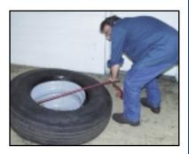
Push tool down to opposite side. First bead is now demounted. Remove tool from wheel. **Do not pick up tire/wheel**.
