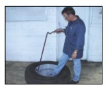
Step through the wheel and pull tool across center of wheel.
