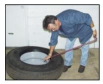
Fully insert **large end** into gap between wheel and tire until you feel bottom bead.
