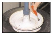
After the tire has been mounted onto the rim and the wheel has been placed onto a tire machine, straighten the bottom bead to lay flat on the rim. Remove the valve core.
