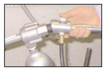
Depress the white button located on top of the bead seater and hold firmly for a few seconds. This allows the cylinder to fill completely. Continue to depress button even after the cylinder is completely filled.
