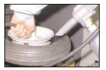
Aim the bead seater nozzle into the opening between the rim and upper bead. For best results, the bead seater nozzle should be pointed into the gap between the rim and the upper bead where the gap is the widest.
