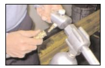
Attach the correct air hose with coupling (80 - 150 psi) to the 1/4" quick disconnect fitting. (The 1/4" male quick disconnect fitting can be purchased from your local hardware store.)
