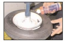
Lubricate the entire bead area before inflating the tire. (Ken-Tool recommends Bead-Eze.) Lubing the tire with a recommended lubricant helps to seal the bead to the rim flange.
