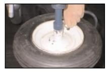
Release the white button to expel the blast of air into the tire. Once the bead is seated, the tire will IMMEDIATELY begin to inflate. STOP inflating when tire is seated to rim. Should a second attempt be necessary, remove the chuck from the tire valve stem and depress white button until cylinder is fully pressurized and repeat steps.
