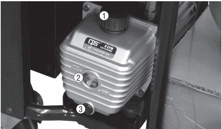
1 - Exhaust / Refill Cap 2 - Oil Sightglass 3 - Oil Drain
