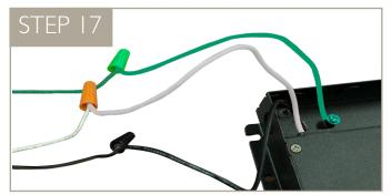
Connect the power supply to AC power/line voltage. Please refer to the wiring diagram of the power supply being used. Each power supply has its own specific wiring.
