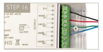
Connect the wires from the RGB LED tape to the output terminals of the receiver. Connect the positive (+) wire to the positive (+) input terminal, and connect the color wires to the corresponding color negative (-) input terminals.
