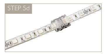
Use the LED-to-LED gripper connector if you are interconnecting LED tape sections. Be sure to align section's positive (+), Red negative (R-), Green negative (G-), and Blue negative (B-) connections.
