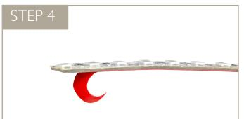
Peel back about a ¼ inch of the red backing and the adhesive tape. Make sure to expose the copper pads on the back of the Linear LED.
