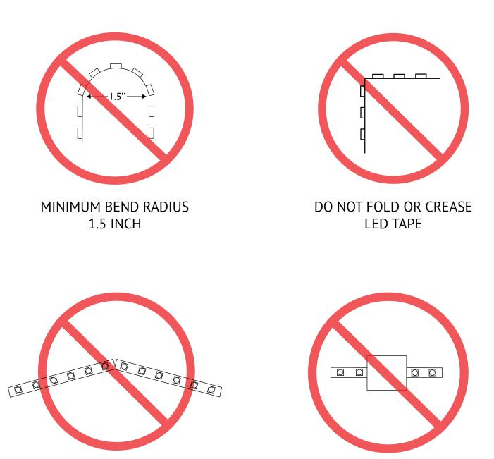
DO NOT BEND LED TAPE SIDE TO SIDE DO NOT COVER LED TAPE OR APPLY EXCESS PRESSURE TO LED TAPE
