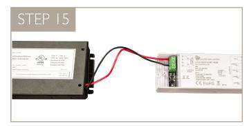
Connect the positive (+) wire from the power supply to the positive (+) input terminal of the receiver. Connect negative (-) wire from the power supply to the negative (-) input terminal of the receiver.
