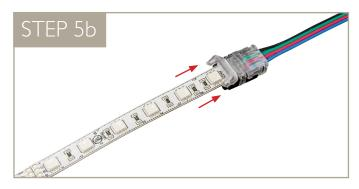
Make note of which wire is positive (+) and which wires correspond to Red negative (R-), Green negative (G-), and Blue negative (B-). Align the LED tape's R-, G-, B-, and positive connections accordingly, then gently push the LED tape into the connector. Be sure to guide the tape over the pins inside the connector.
