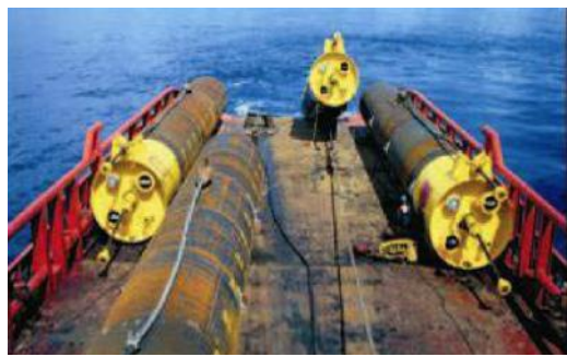
Suction type anchors.
